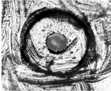
Figure 5-6. Damage from improper cleaning.
